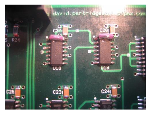
The picture above shows these jumpers installed on the board. The picture on the following page shows the completed divider.
